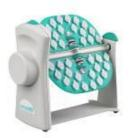
To create a Tumbling motion for your samples, turn the Rotisserie plates so the samples are in a "Vertical Mixing Position"
